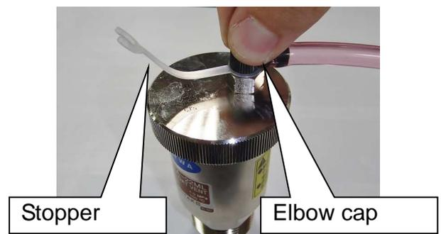
10. Since elbow cap is made of resin, it is treated as consumable supply.
