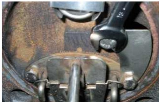
After temporarily tightening the three bolts, tighten them with torque of 30 N·m with a torque wrench (width across flat: 13 mm).
