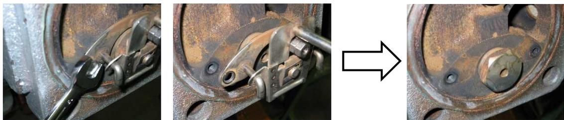
[Procedure 7] Remove the valve seat with socket wrench (width across flat: 39 mm).
