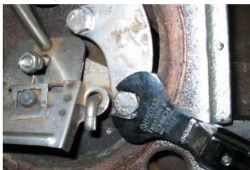
[Procedure 6] Put a new gasket on the cover and tighten the hexagon bolts and nuts fixing the body with 200 N·m torque using torque wrench (width across flat: 32 mm).
