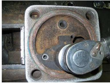
[Procedure 2] Assemble the air vent valve seat, air vent cover and air vent gasket, and attach them to the cover by tightening with 50 N·m torque using torque wrench (width across flat: 19 mm). At that time, adjust the air vent cover to make its rectangular holes come on both sides (not top and down), as shown in the picture.
