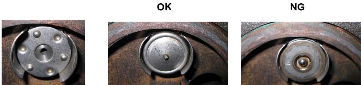
[Procedure 4] Air vent holder can be assembled by hand.
