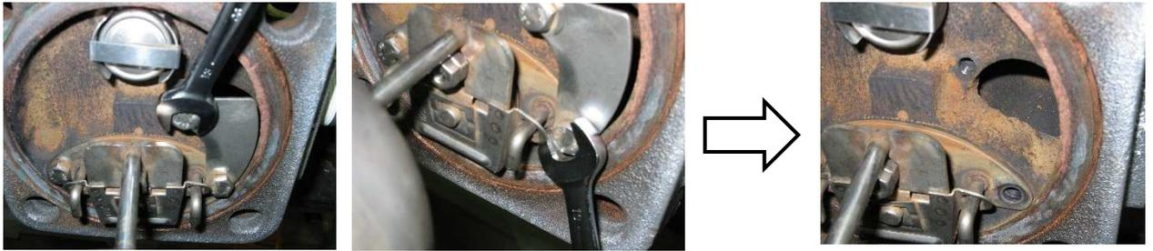
[Procedure 6] Remove the hexagon bolt on the outlet side of the float holder with spanner, ring wrench, etc (width across flat: 13mm). Then the float (P) and float holder can be removed. The valve is attached to the float (P).
