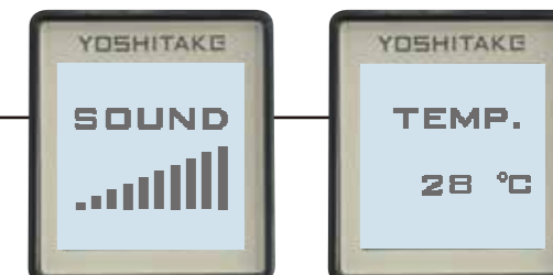
Auscultation or surface temperature measurement only is possible by easy switching operation.
