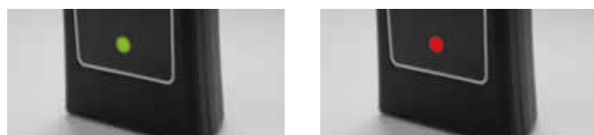
LED shows diagnosis result by different colors (green, yellow, or red).
