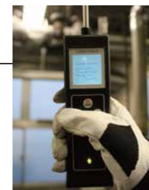
Auscultation or surface temperature measurement only is possible by easy switching operation.
