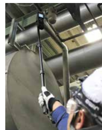
Extensible bar (to be prepared by customers) for inspections at high, distant or narrow spaces.
